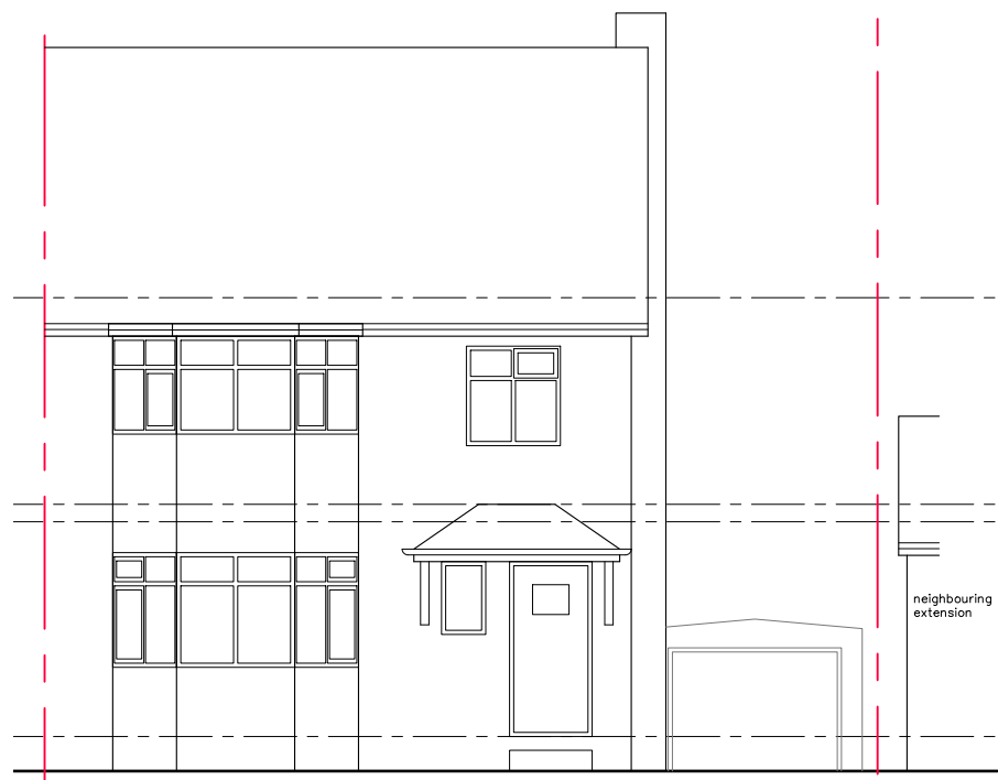
Existing North (front) Elevation 1:100
